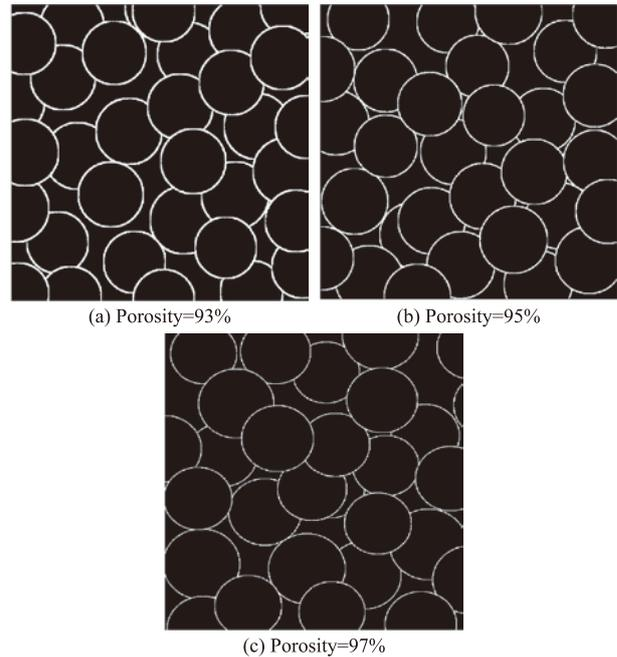
Fig.4 Reconstructed microstructures with different porosity
