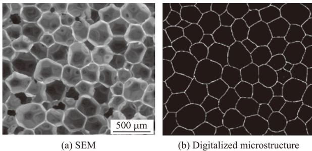
Fig.2 SEM of polyurethane foam (a) and its digitalization (b)
