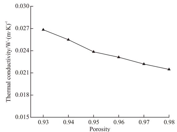
Fig.5 Effective thermal conductivity varied with the porosity
