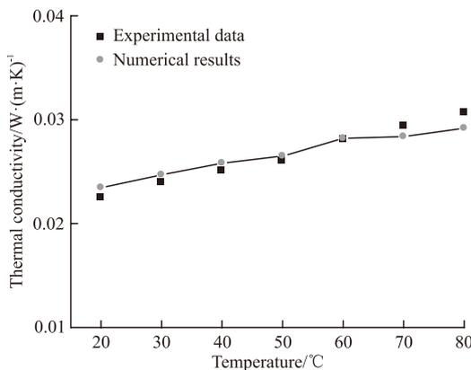
Fig.3 Comparisons of the numerical results and experimental data
