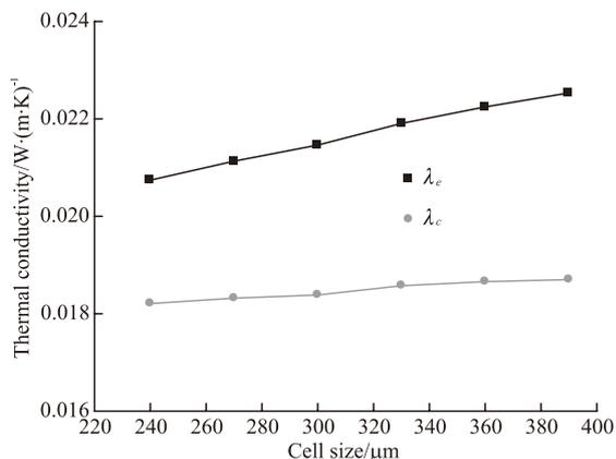
Fig.7 Effective thermal conductivity varied with the cell size
