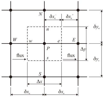
Fig.1 Grid system in Cartesian coordinates
