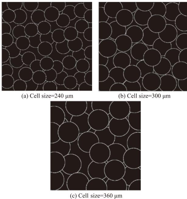
Fig.6 Reconstructed microstructures with different porosity
