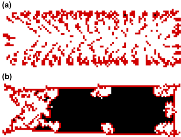
Fig. 3. The final geometries of the primary phase ( D_{(s)} ) and the secondary phase ( P_{(s)} ) under different crystal growth mechanisms: (a) concentration-controlled precipitation and (b) epitaxial precipitation. The dissolving primary phase is black and the precipitating secondary phase is red. The values of all the parameters are the same as those in Figure 1.
