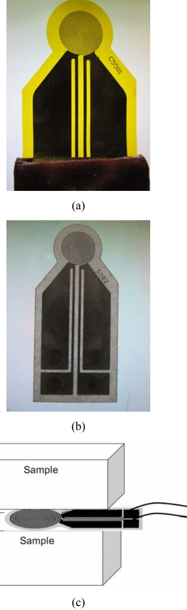
Figure 1 Sensor shape and test sample arrangement, (a) kapton5501 sensor (b) mica5082 sensor (c) sandwich structure (see online version for colours)
