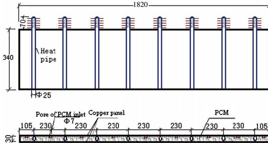
Fig. 15. The re-constructed shelf 4 with heat pipes and PCM.
