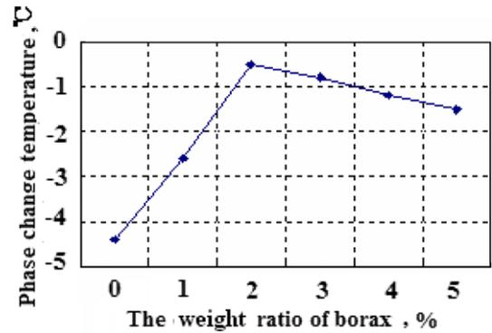
Fig. 14. The phase change temperature of PCM.
