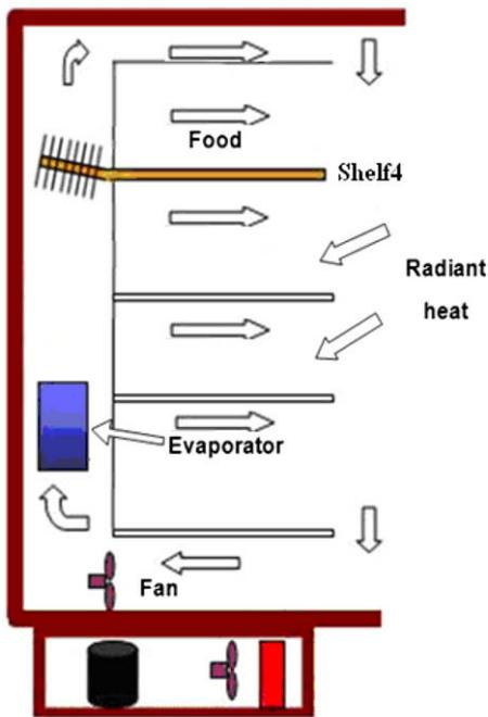
Fig. 8. A typical multi-deck type display cabinet with heat pipes.
