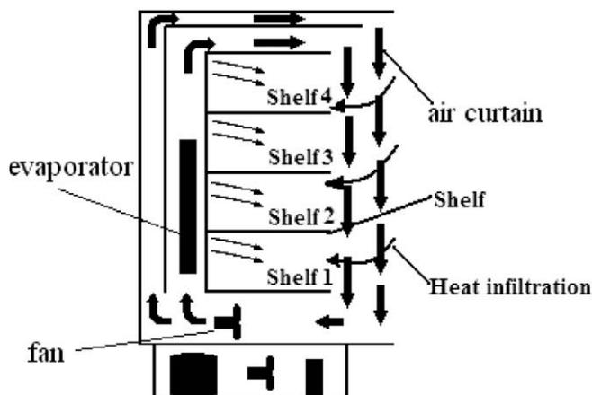
Fig. 1. Schematic of a conventional display cabinet.
