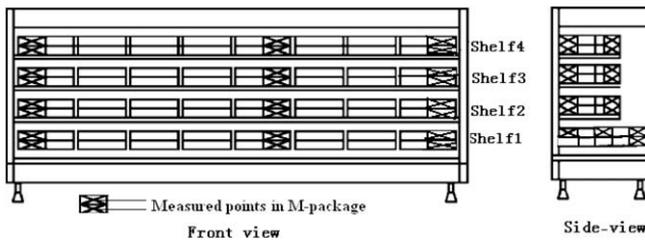
Fig. 5. The experimental points measured in conventional cabinet.
