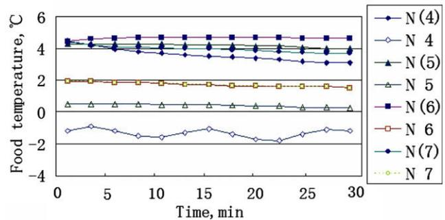
Fig. 10. Food temperatures on the same position with and without heat pipes (N4-7).
