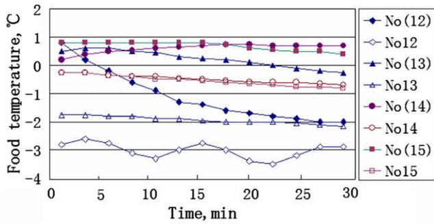
Fig. 12. Food temperatures on the same position with and without heat pipes (N12–15).
