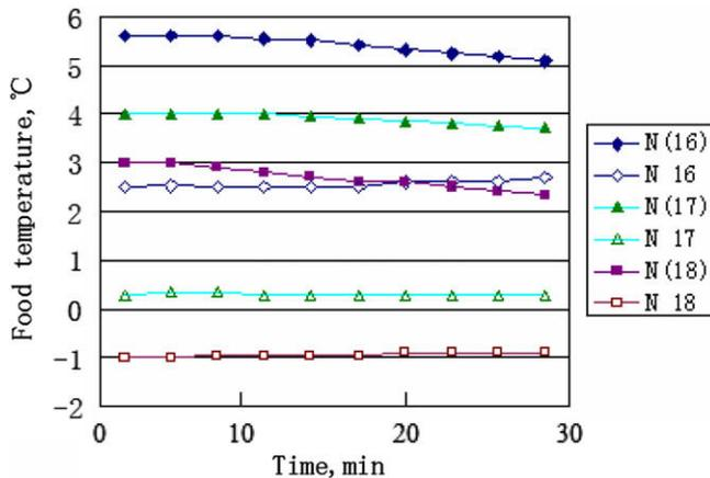
Fig. 13. Food temperatures on the same position with and without heat pipes (N16–18).
