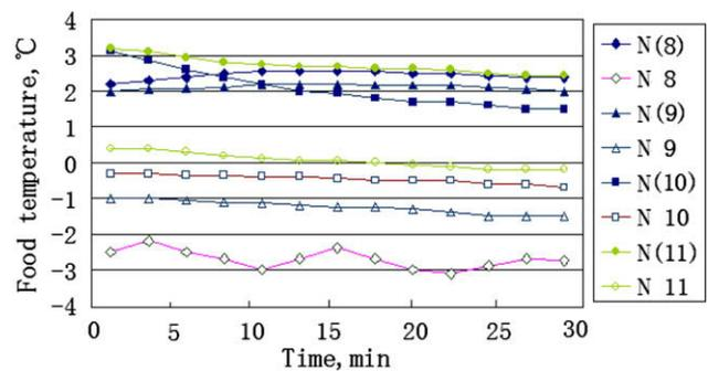
Fig. 11. Food temperatures on the same position with and without heat pipes (N8-11).
