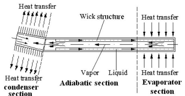
Fig. 7. Principle of operation of a heat pipe.
