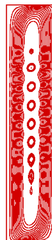
Figure 3 Streamline pattern calculated with QUICK + TFQMR ( 32 \times 145 ) (see online version for colours)
