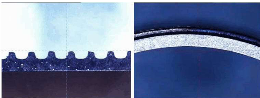
Fig. 2. Geometric structure of enhanced titanium tube.
