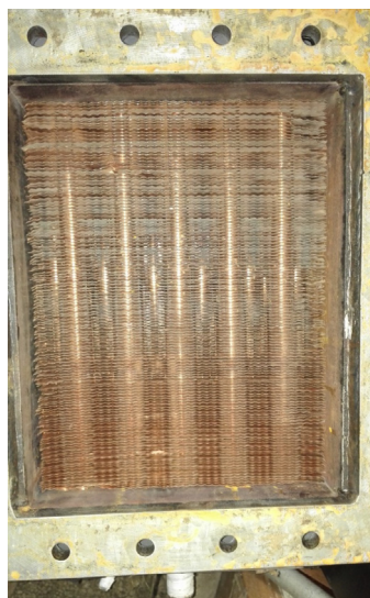
(b) Cross section of test heat exchanger
