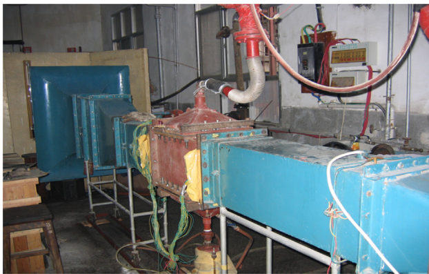
(a) Heat transfer wind tunnel without thermal insulation
