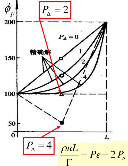
Thus when  $P_{\Delta}$  is larger than 2, numerical solutions are unrealistic (不现实的):  $\phi_P$  is less than its two neighboring grid values, which is not possible for the case without source.
