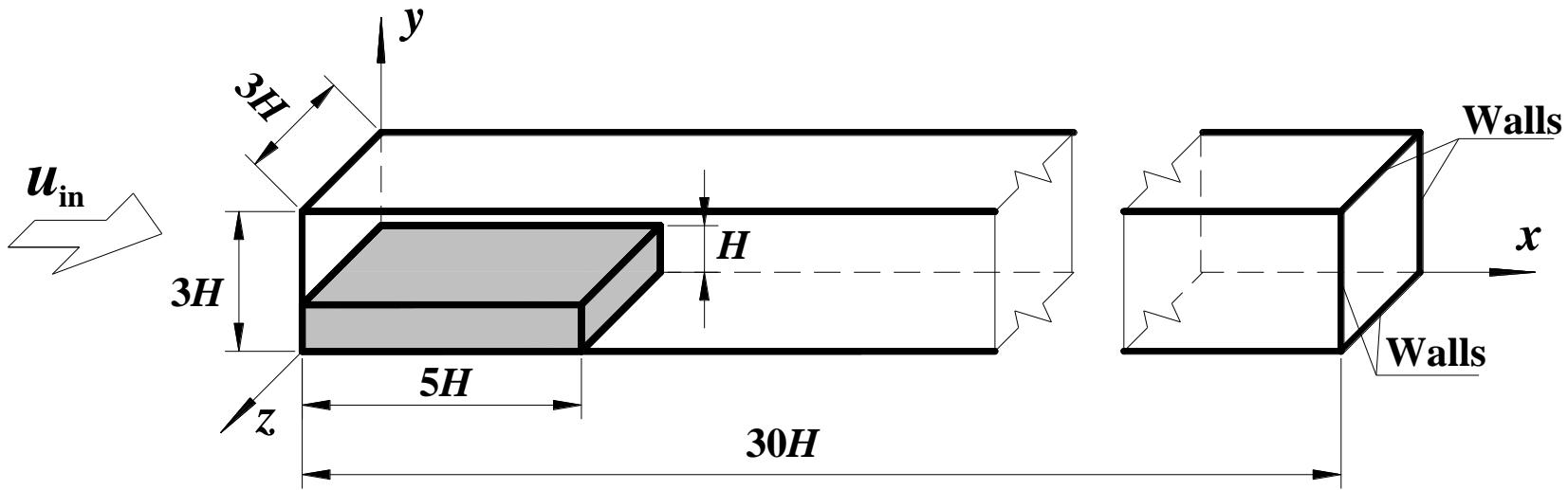
Flow configuration of laminar fluid flow
