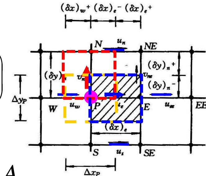
$$\left\{ \begin{array}{l} a_e u_e = \sum a_{nb} u_{nb} + b + (p_P - p_E) A_e \\ a_n v_n = \sum a_{nb} v_{nb} + b + (p_P - p_N) A_n \\ [(\rho u)_e - (\rho u)_w] \Delta y + [(\rho v)_n - (\rho v)_s] \Delta x = 0 \end{array} \right.$$
