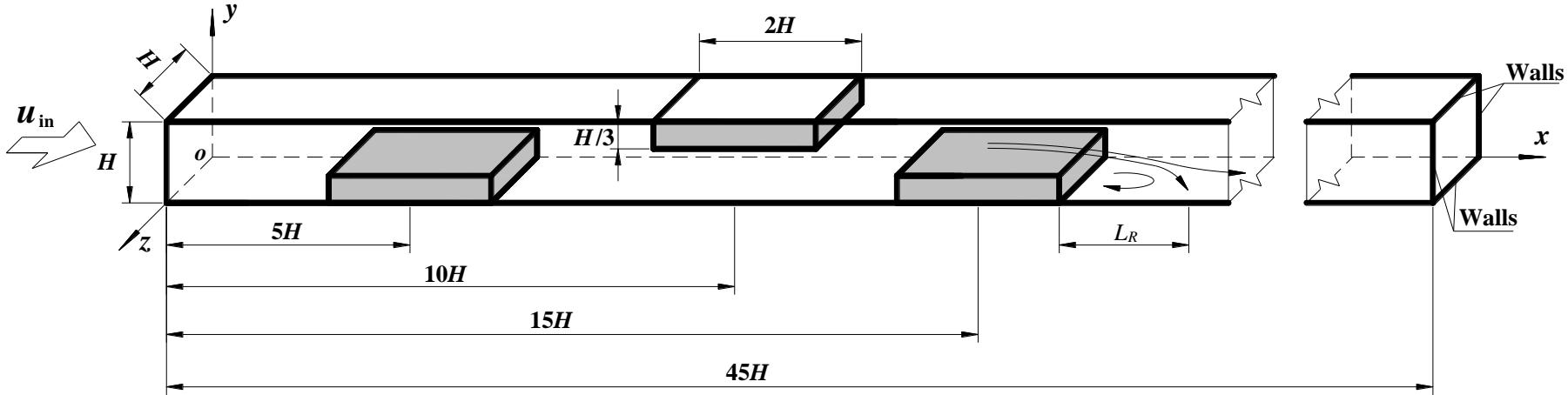
Flow configuration of laminar fluid flow through a 3-D duct with complicated structure
