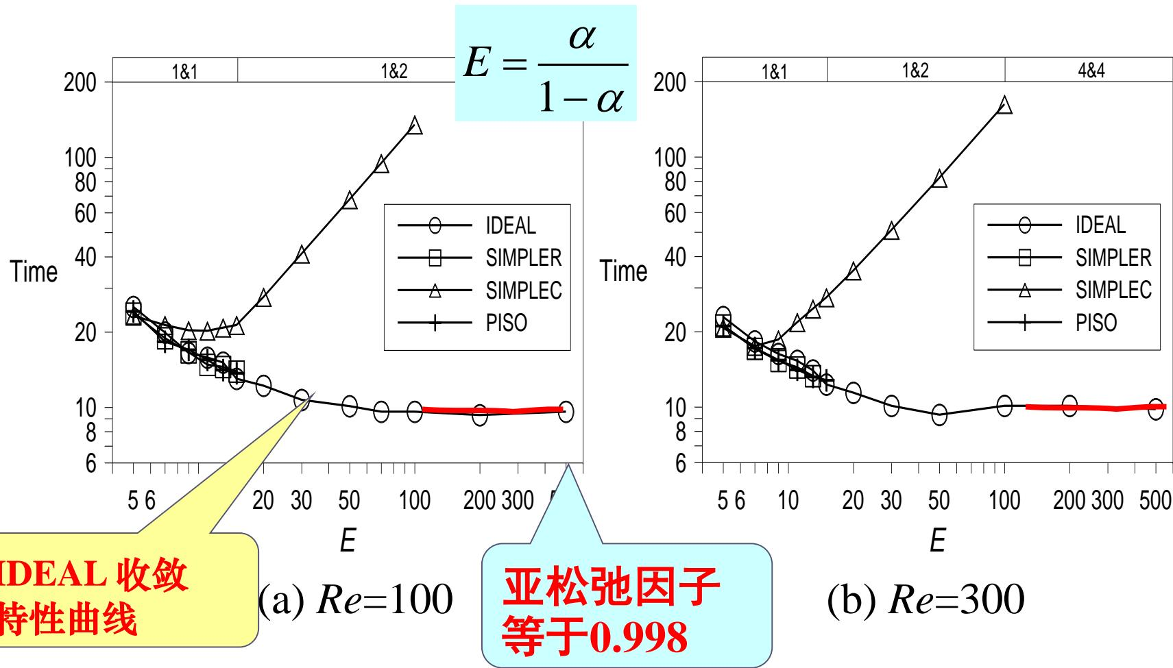
Comparison of computation time and robustness of IDEAL, SIMPLER, SIMPLEC and PISO algorithms for (a)  $Re=100$  and (b)  $Re=300$  with grid number= $32 \times 32 \times 32$
