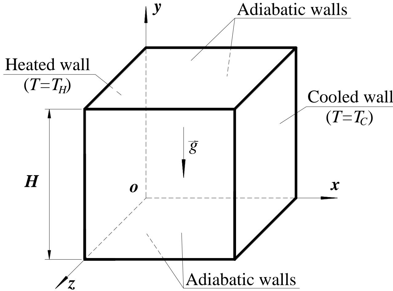
Flow configuration of natural convection in a cubic cavity
