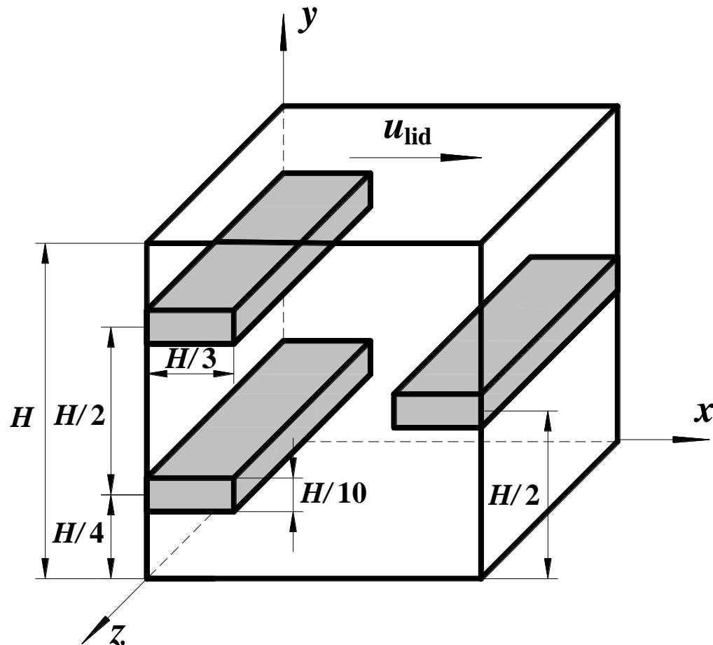
Flow configuration of lid-driven cavity flow in a cubic cavity
