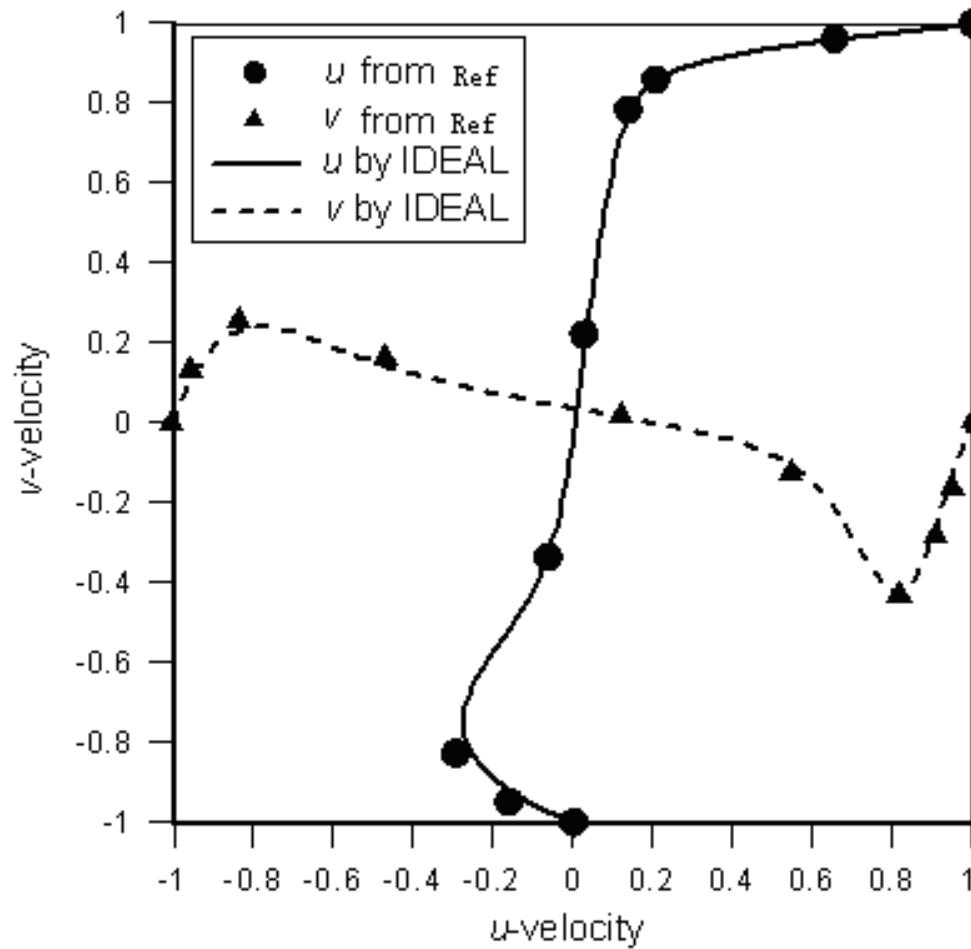
Comparison of velocity profiles  $u$  and  $v$  along the central axes
