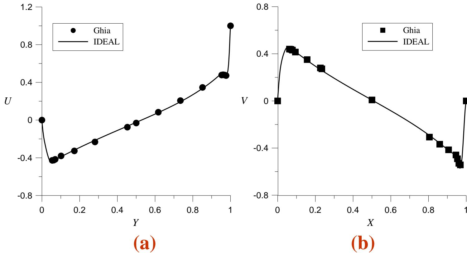
**Fig. Predicted velocity distributions for  $Re=10000$  and grid numbers= $260 \times 260$**
