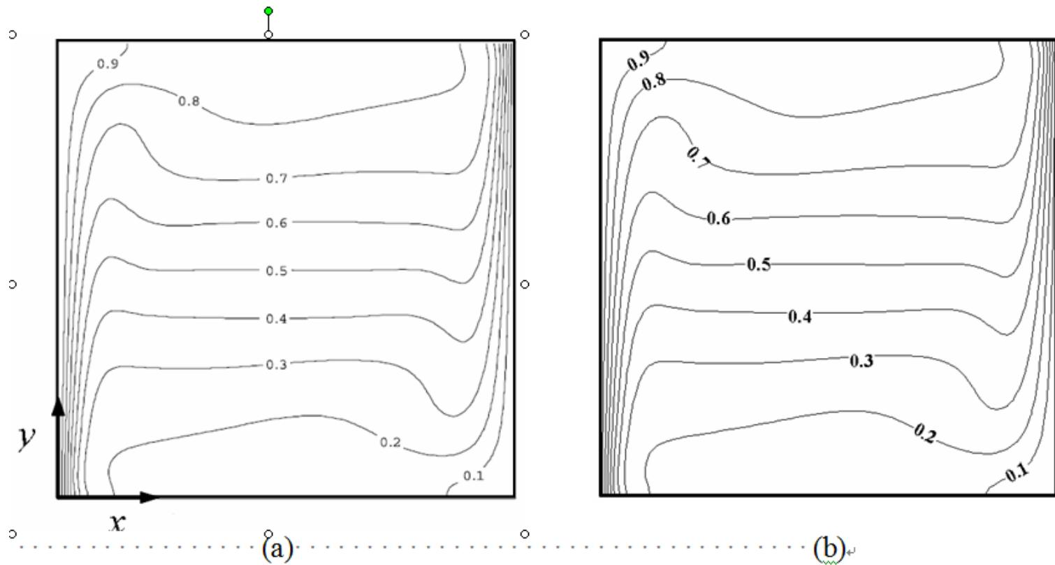
Temperatures at the plane  $z=0.5H$  for  $Ra=10^6$ , obtained
