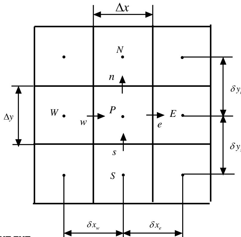
Fig. 2-D staggered grid
