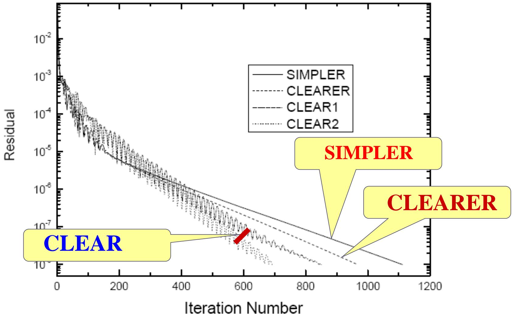
They attributed the oscillation of the numerical solution during iteration to the fact that in SIMPLER the revised velocity is composed of two parts: a major part—intermediate velocity  $u^*, v^*$  and the minor part—corrections  $u', v'$ ,
