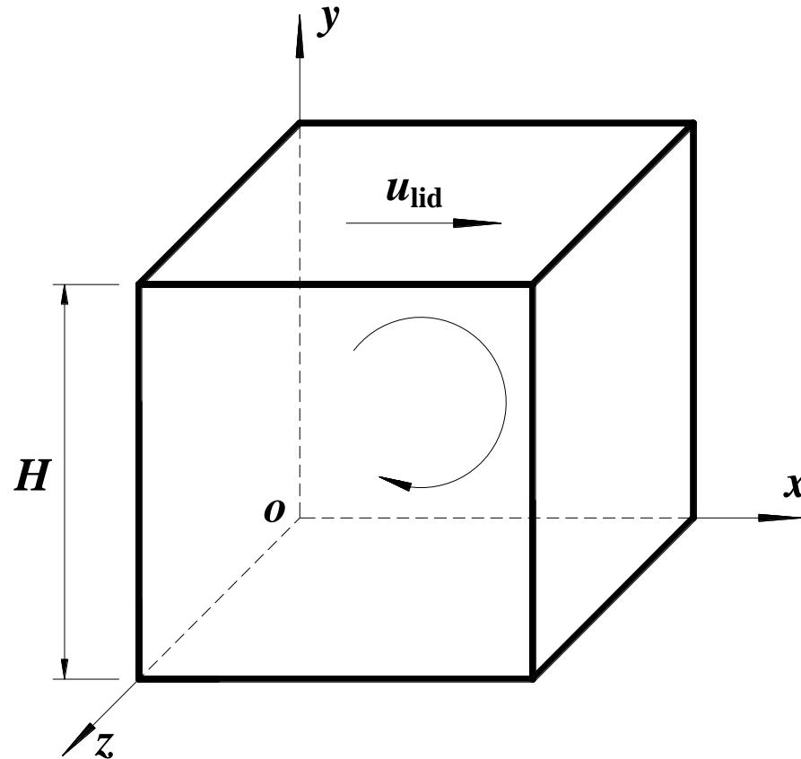
Flow configuration of lid-driven cavity flow in a cubic cavity
