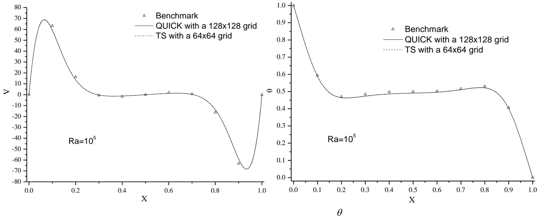
**V velocity and dimensionless temp. along the center vertical line of the cavity at  $Ra=10^5$  (64X64 for S-T vs. 128X128 for QUICK)**
