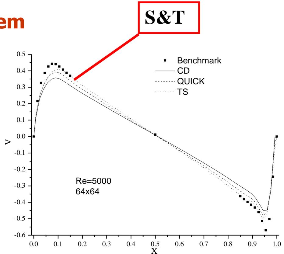
Computed velocity along the line passing through the geometric centre of the cavity at  $Re=5000$ ,  $64 \times 64$  grid system.
