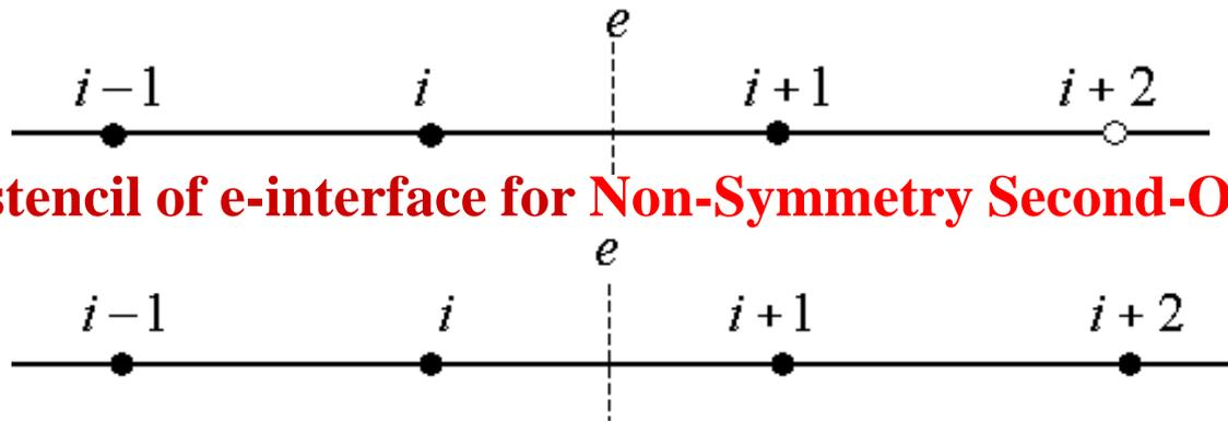
Four-grid stencil of e-interface for Non-Symmetry Second-Order(QUICK)
