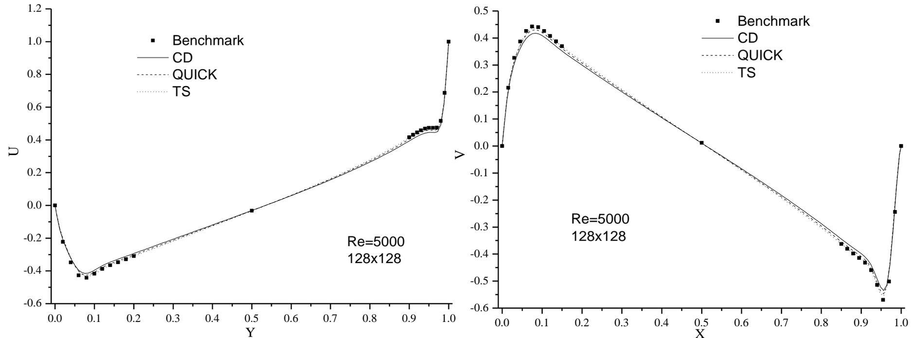
**Computed velocity along the line passing through the geometric centre of the cavity at Re=5000, 128x128 grid system.**
