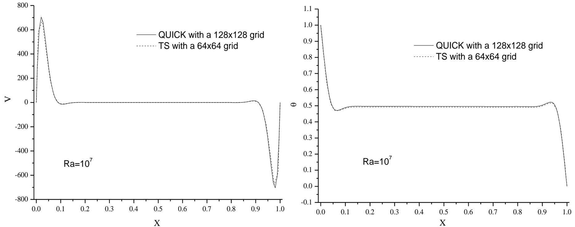
**Fig.  $V$  velocity and dimensionless temp. along the center vertical line of the cavity at  $Ra=10^7$**
