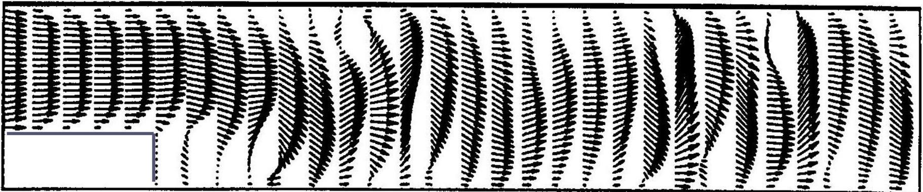
Figure Velocity vector using QUICK ( $Re=300$ ,  $Er=1.5$ ,
