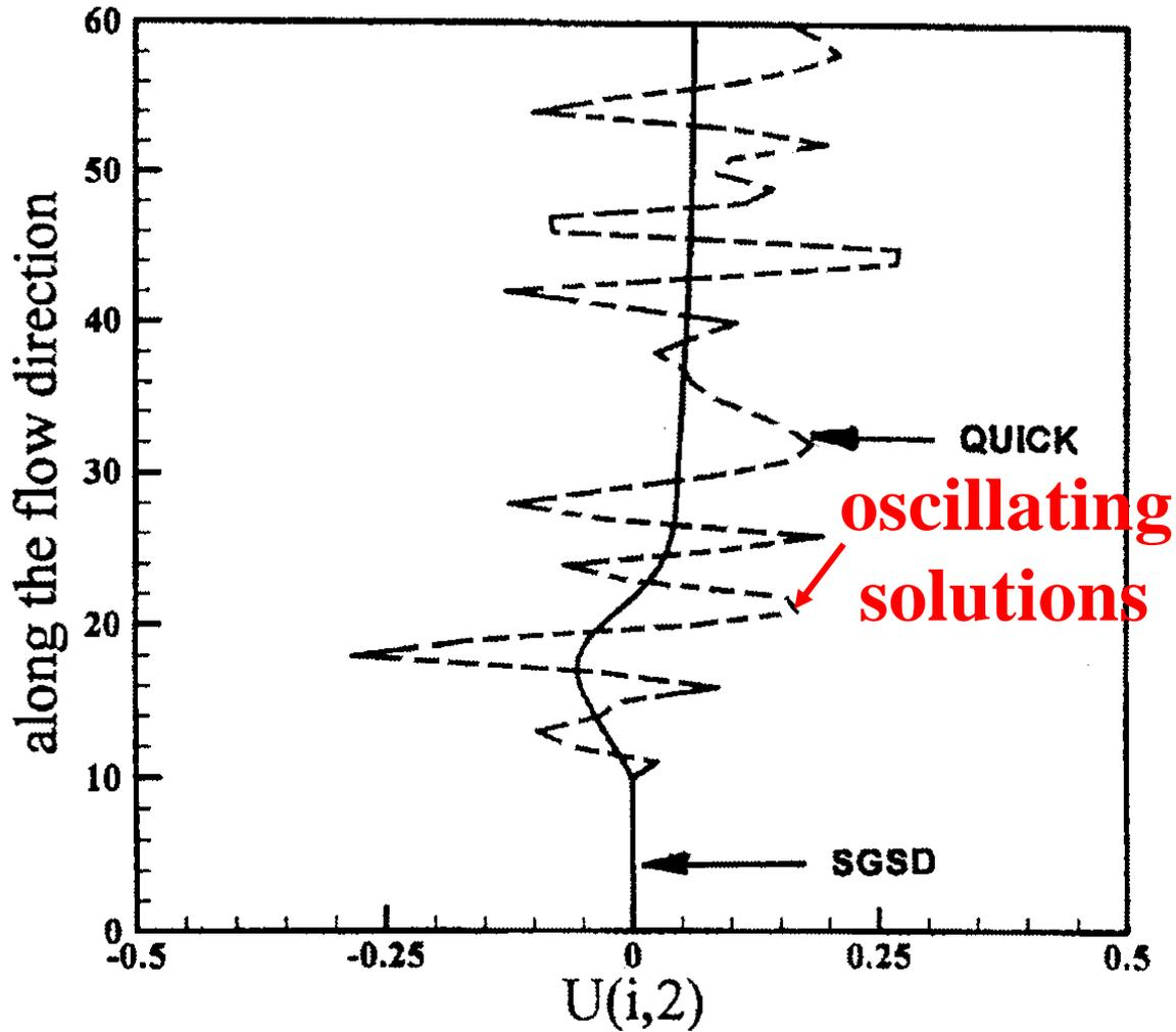
Velocity distribution along the grid line parallel to the bottom
