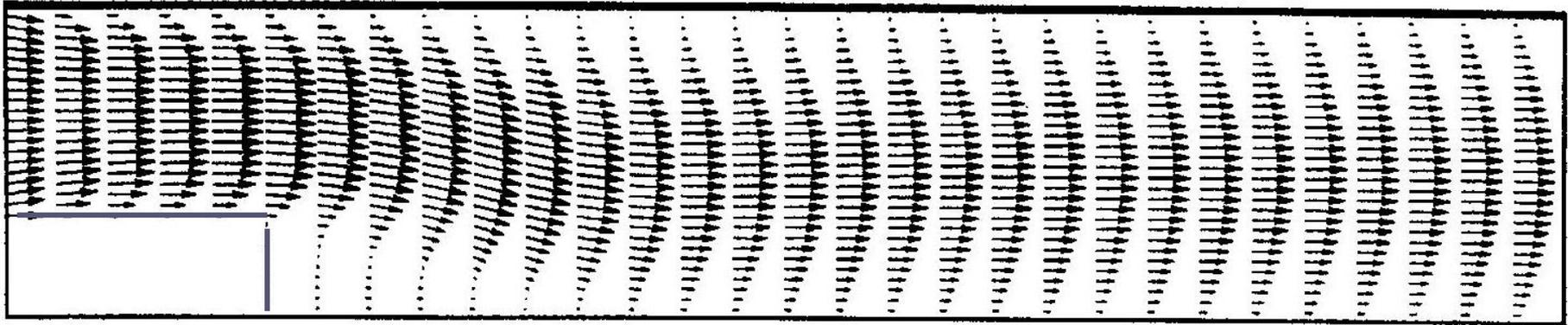
Figure Velocity vector using SGSD ( $Re=300$ ,  $Er=1.5$ ,
