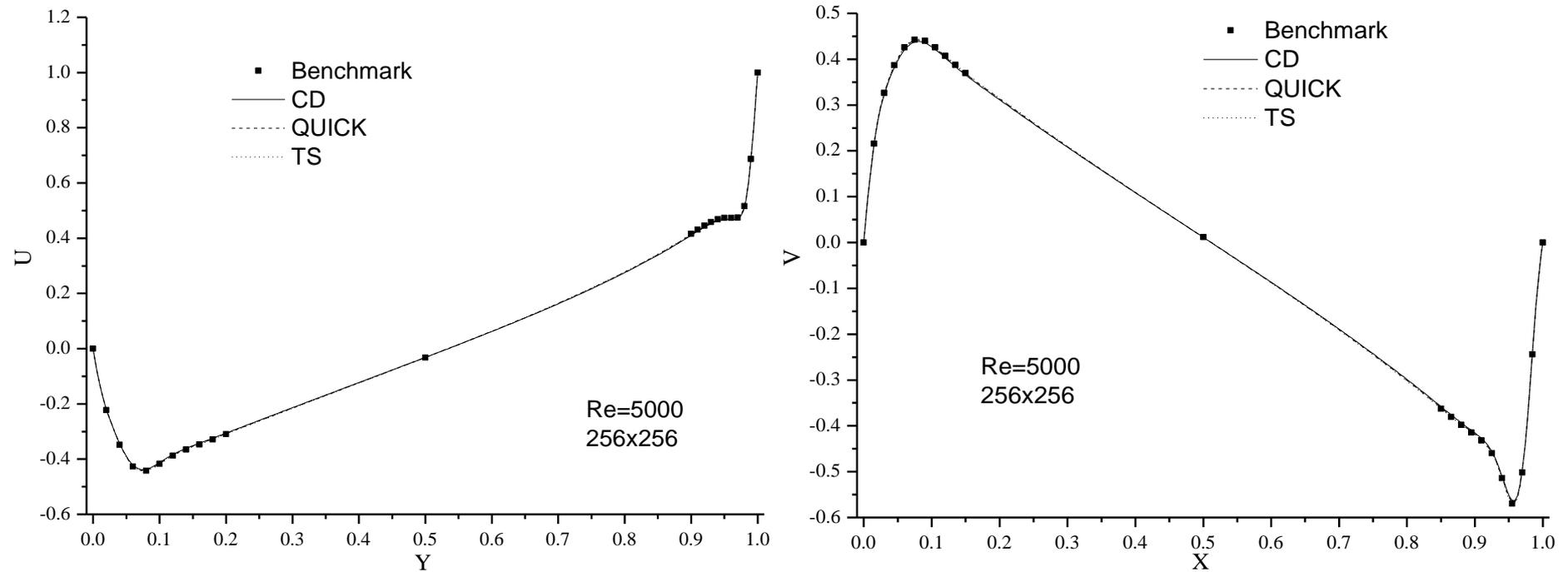
**Computed velocity along the line passing through the geometric centre of the cavity at Re=5000, 256x256 grid system.**
