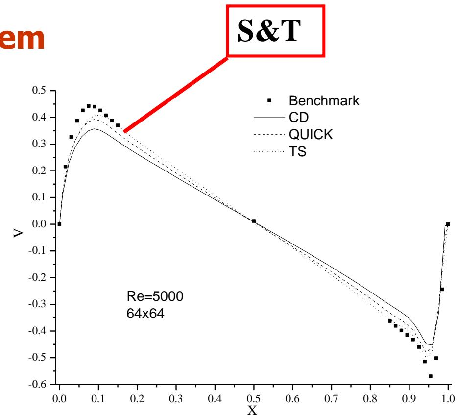
Computed velocity along the line passing through the geometric centre of the cavity at Re=5000, 64x64 grid system.
