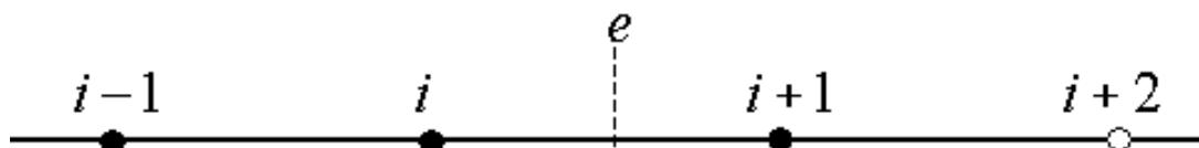
Four-grid stencil of e-interface for Non-Symmetry Second-Order(QUICK)
