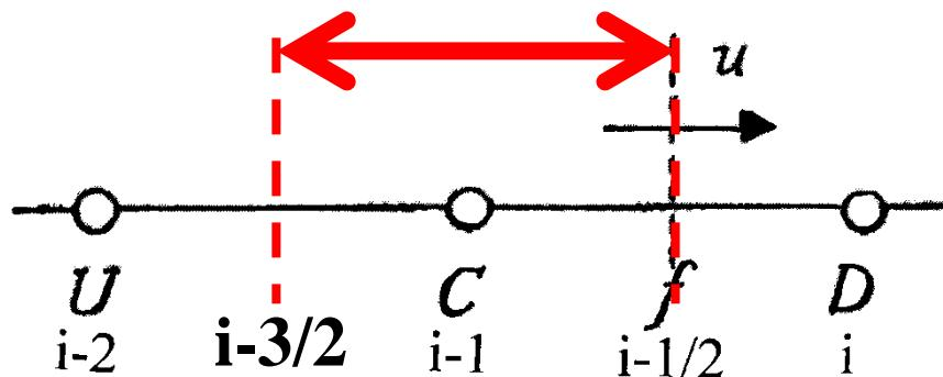
$$\rho u (\phi_{i-1/2} - \phi_{i-3/2}) = (\Gamma \frac{d\phi}{dx})_{i-1/2} - (\Gamma \frac{d\phi}{dx})_{i-3/2} + \int_{i-3/2}^{i-1/2} S_\phi dx$$
