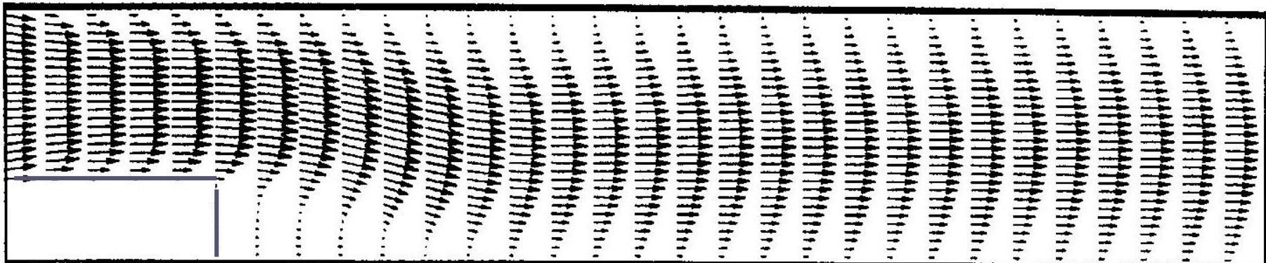
**Figure Velocity vector using SGSD (Re=300, Er=1.5,
