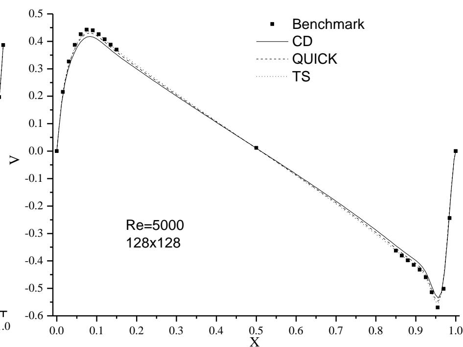
Computed velocity along the line passing through the geometric centre of the cavity at  $Re=5000$ ,  $128 \times 128$  grid system.
