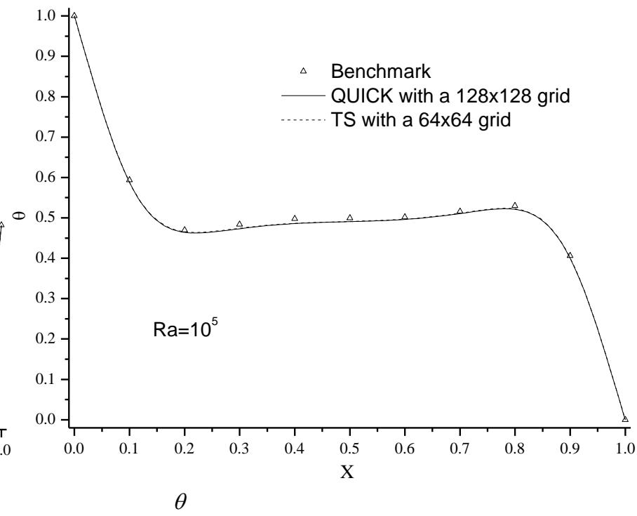
**V velocity and dimensionless temp. along the center vertical line of the cavity at  $Ra=10^5$ (64X64 for S-T vs. 128X128 for QUICK)**
