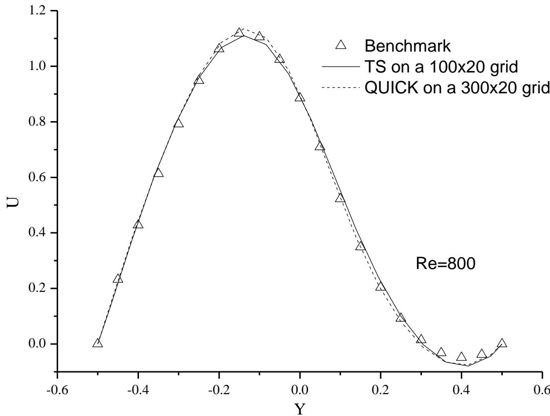
Computation on a grid of 100X20 by QUICK can not reach converged solutions . A 300 X20 grid must be used for QUICK
