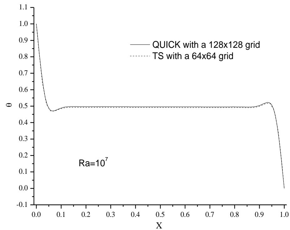
**Fig. V velocity and dimensionless temp. along the center vertical line of the cavity at  $\text{Ra}=10^7$**
