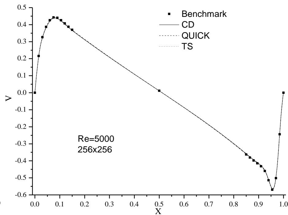
**Computed velocity along the line passing through the geometric centre of the cavity at Re=5000, 256x256 grid system.**
