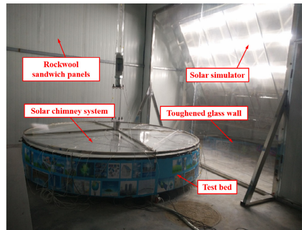
(a) System A: the solar chimney system
