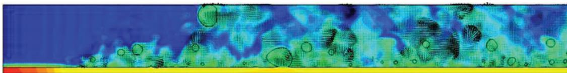
Fig. 12. Velocity distribution at the central section of the mini-channel with a heat flux of  $400 \text{ kW/m}^2$  at 100 ms.
